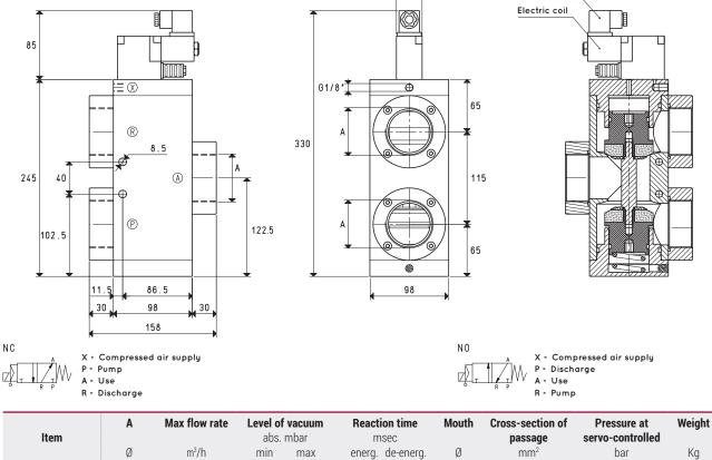
0.5 Note: The coil and the connector are not integral parts of the solenoid valve and, therefore, must be ordered separately (See accessories for solenoid valves). Solenoid valve servo-controlled power must be supplied with non-lubricated compressed air, 5 micron filtration, according to standard ISO 8573-1 class 4.
